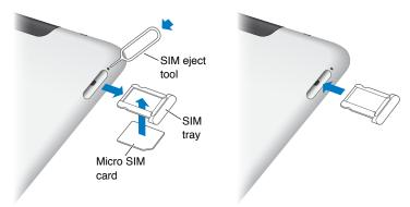
Open the SIM tray: Insert the tip of the SIM eject tool into the hole on the SIM tray. Press firmly and push the tool straight in until the tray pops out. Pull out the SIM tray to install or replace the SIM card. If you don't have a SIM eject tool, you may be able to use the end of a small paper clip.
